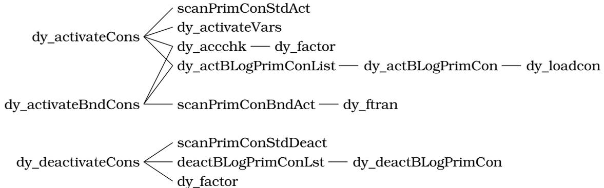
Figure 14: Call Graph for Constraint Management Routines
