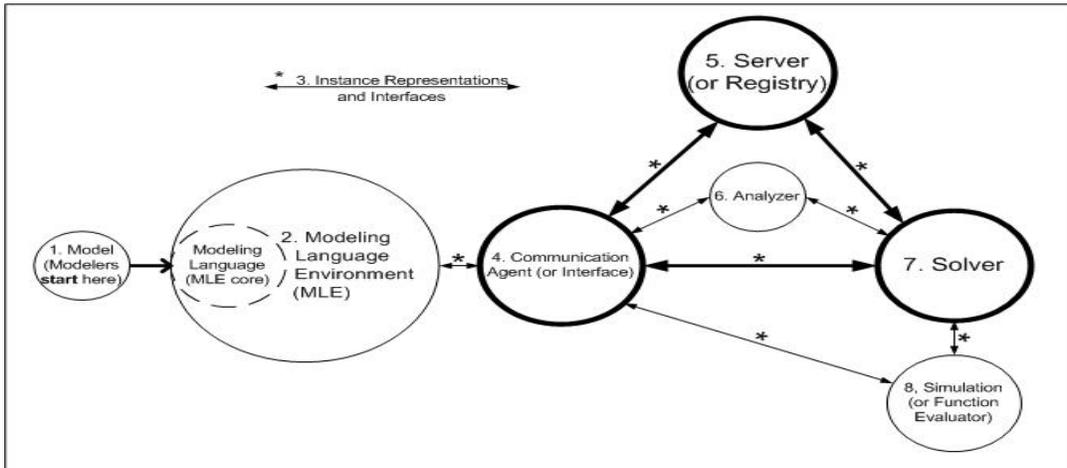
**Figure 2-1: A typical optimization system and component interaction.**
