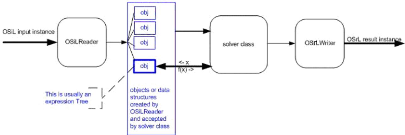
**Figure 2-3: A generic input and output process of an Optimization Services compatible solver.**
