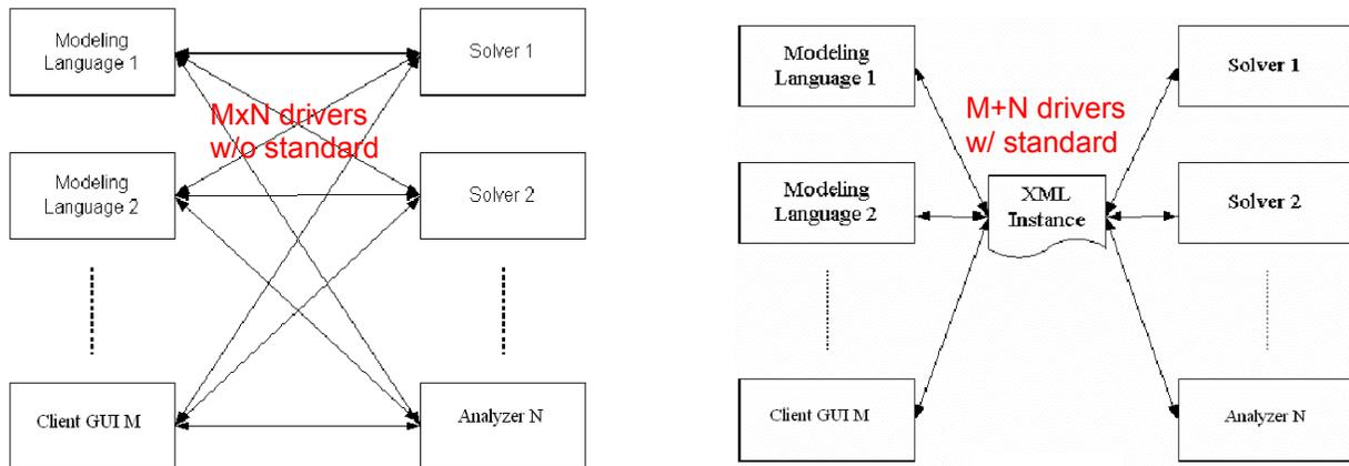
**Figure 1-5:  $M+N$  drivers needed by  $M$  modeling languages (or GUIs) and  $N$  solvers (or analyzers) with a standard XML instance.**
